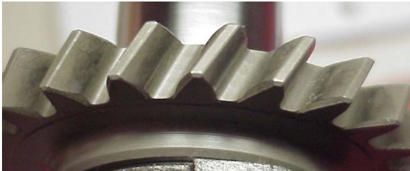
Tight mesh-capable, low contact ratio
