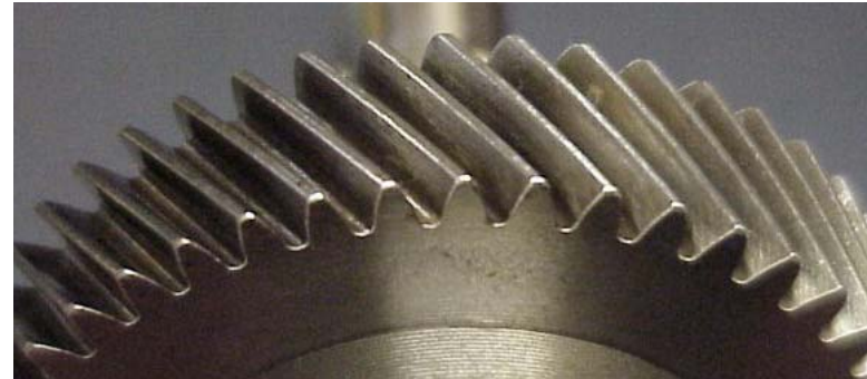
NVH-robust high contact ratio
